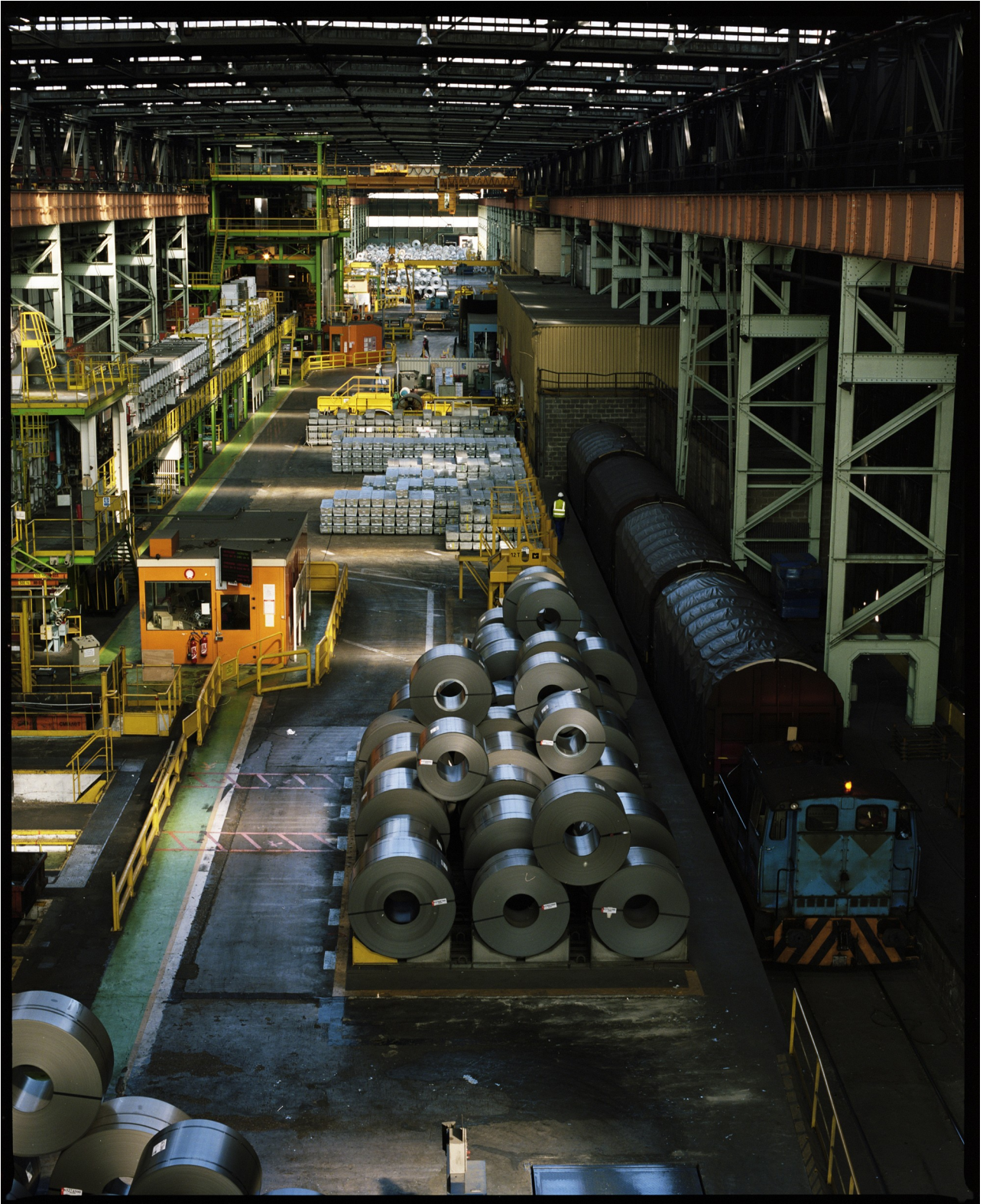
Arcelor-Mittal factory, Route de Saint-Leu, Montataire. Galvanised and lacquered sheet steel production line.
